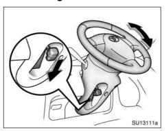
To change the steering wheel angle, hold the steering wheel, push down the lock release lever, tilt the steering wheel to the desired angle and return the lever to its original position.
