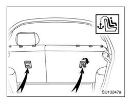
Open the anchor bracket cover with the symbol mark shown in the illustration.
