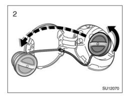
To remove the fuel tank cap, turn the cap slowly counterclockwise, then pause slightly before removing it. After removing the cap, hang the tether as shown in the illustration.
