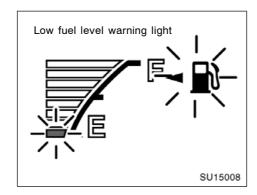
If the low fuel level warning light flashes, fill the fuel tank as soon as possible.
