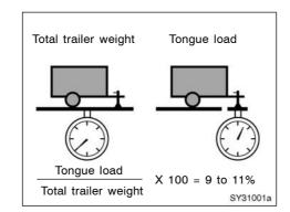
● The trailer cargo load should be distributed so that the tongue load is 9 to 11% of the total trailer weight, not exceeding the maximum of 31 kg (68 lb.). Never load the trailer with more weight in the back than in the front. About 60% of the trailer load should be in the front half of the trailer and the remaining 40% in the rear.
