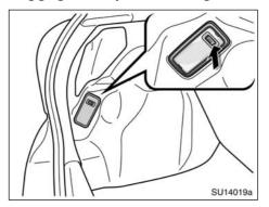
To turn the luggage compartment light on, open the back door and push the switch to right. Closing the back door will turn the light off.
