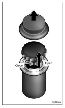
Check the fluid level through the reservoir. If necessary, add automatic transmission fluid DEXRON®II or III.
