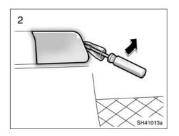
Remove the front towing eyelet cover on the front bumper, using a flatbladed screwdriver which is wrapped with a cloth.
