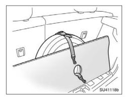
Put the spare tire cover against the flat tire, and then pass the rest of the belt hooks thorough the hole in the cover.
