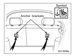
Use the anchor bracket behind the rear seat to attach the top strap.
