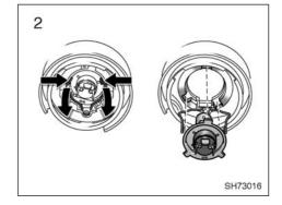
Release the bulb retaining spring and remove the bulb. Install a new bulb and the bulb retaining spring.
