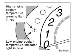
The indicator and warning lights indicate the engine coolant temperature when the ignition switch is on. The engine operating temperature will vary with changes in weather and engine load.
