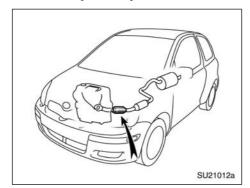
The three-way catalytic converter is an emission control device installed in the exhaust system.
