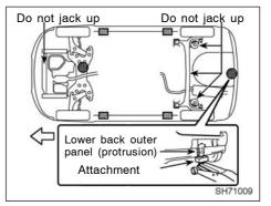
When jacking up your vehicle with the jack, position the jack correctly as shown in the illustration.
