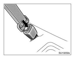
4. To remove the convertible seat, press the buckle release button and allow the belt to retract completely. The belt will move freely again and be ready to work for an adult or older child passenger.
