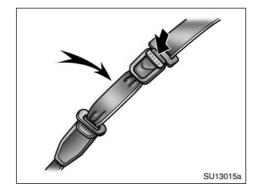
To connect the extender to the seat belt, insert the tab into the seat belt buckle so that the "PRESS" signs on the buckle release buttons of the extender and the seat belt are both facing outward as shown.
