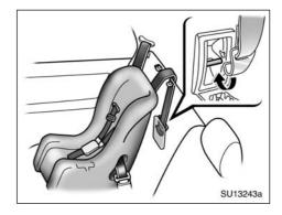
Securely fasten the child restraint system with the seat belt.
