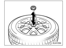
Aluminum wheels—Before stowing the flat tire, remove the center wheel ornament.
