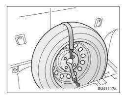
Place a flat tire against the seatback with the tire in an upright position.
